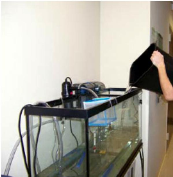
13. Plug in all electric cords using the power strip, but keep the power off. Once everything is plugged in, stand back from the tank to double check all connections and ensure that everything is ready for operation. The output tube should be secure; a student can hold this tube in place. Have some paper towels on hand in the event of a leak.
